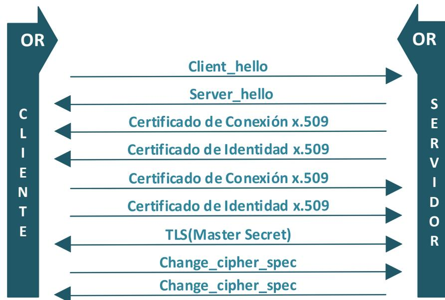
Figura 12. Handshake version 1 – Certificates up front
