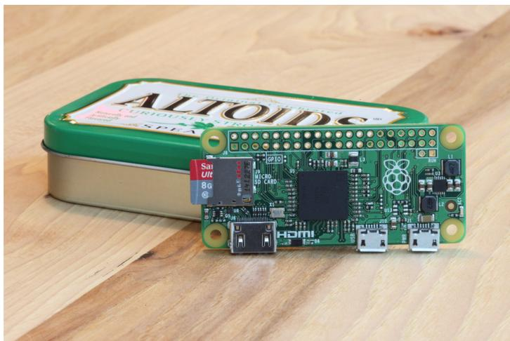
Figura 6: Raspberry-Pi Zero
